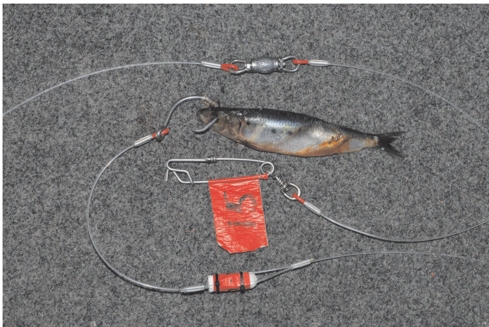
Figure 3. Branch line showing 60 g leaded swivel, bait, hook type and position in bait, mainline clip and location of time-depth recorders used in the experiment.
