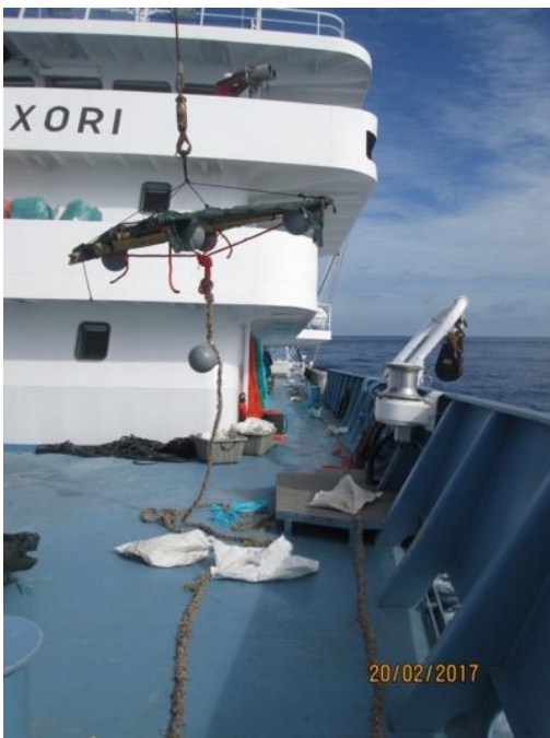
Figure 3. FAD type 2: A single rope hanging from the center of the raft. This design was used at 30 m 50 m and 70m depth.
