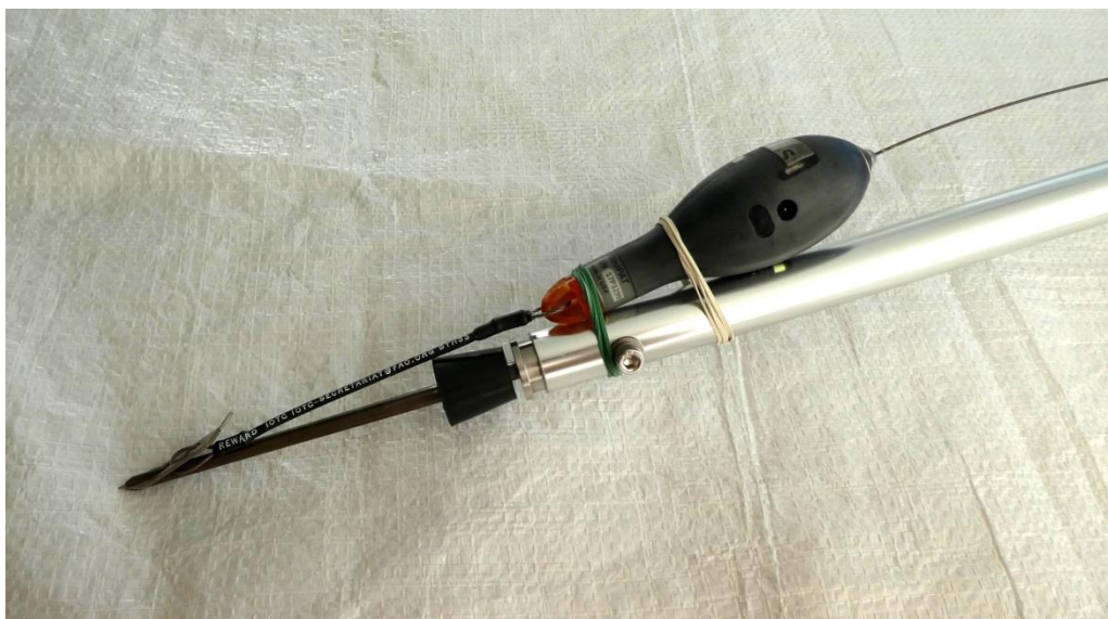
Figure 8. Mounting of tag on a tagging pole. Upper panel (A, B): attachment of anchor to applicator; Lower panel (C): attachment of tag to tagging pole with rubber bands.
