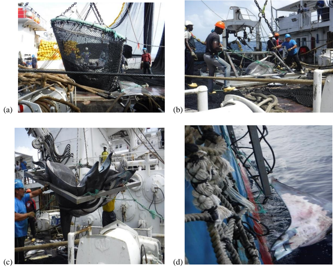
Figure 4. AZTI manta sorting grid use release steps: (a) empty bail contents into unloading hatch, (b) connect grid frame with chains to deck crane, (c) move sorting grid towards starboard railing, and (d) release animals into the water.
