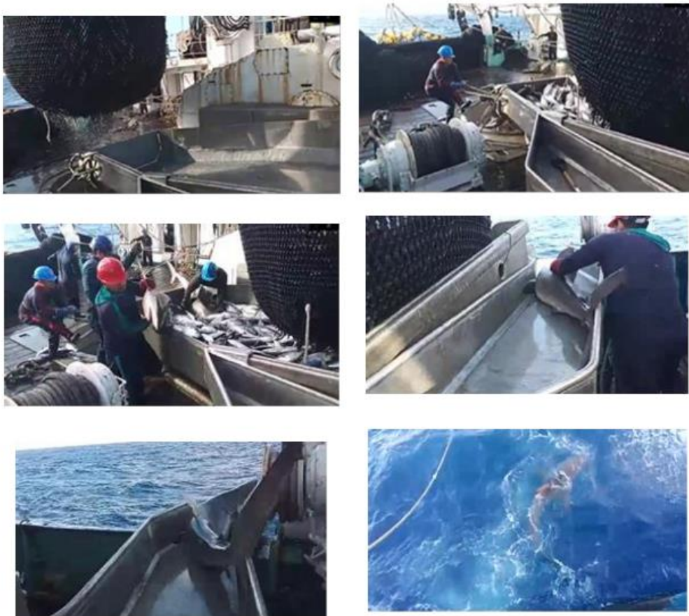
Figure 8. Sequence of brailing and shark release using hopper with ramp in the top deck on the starboard.
